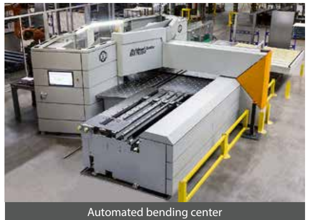
Metal forming line of skeleton rails
