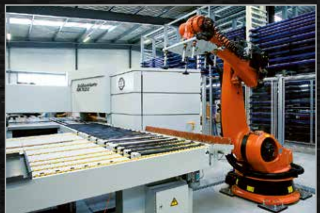
Automated bending center
