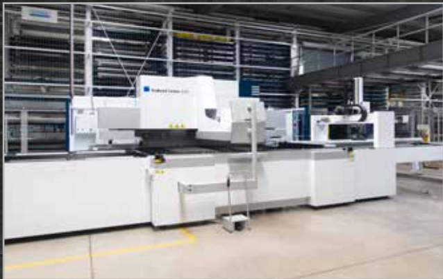
Automated bending center
